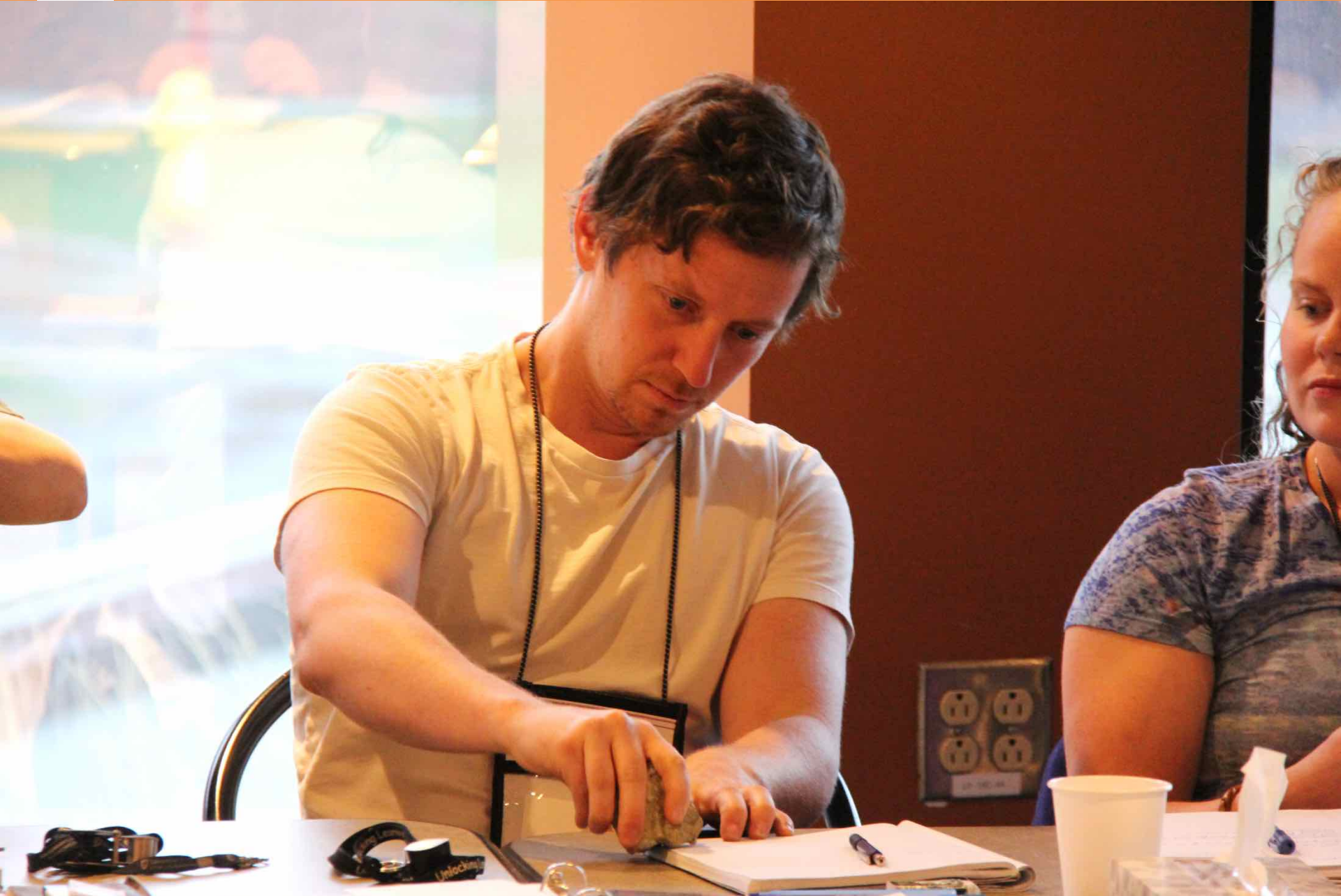
Jeremy Beales (U Vic) identifies chalcocite in his sample after performing a streak test
