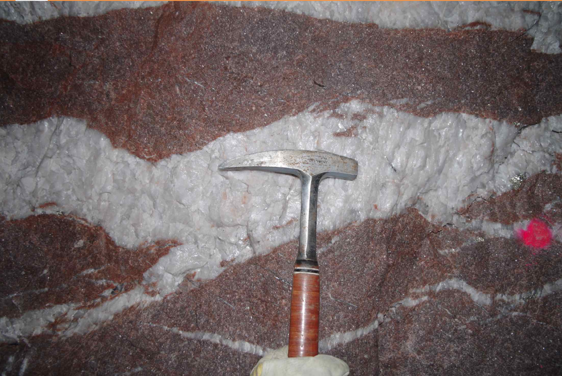
Syenite-hosted auriferous quartz veins in the Timmins West mine
