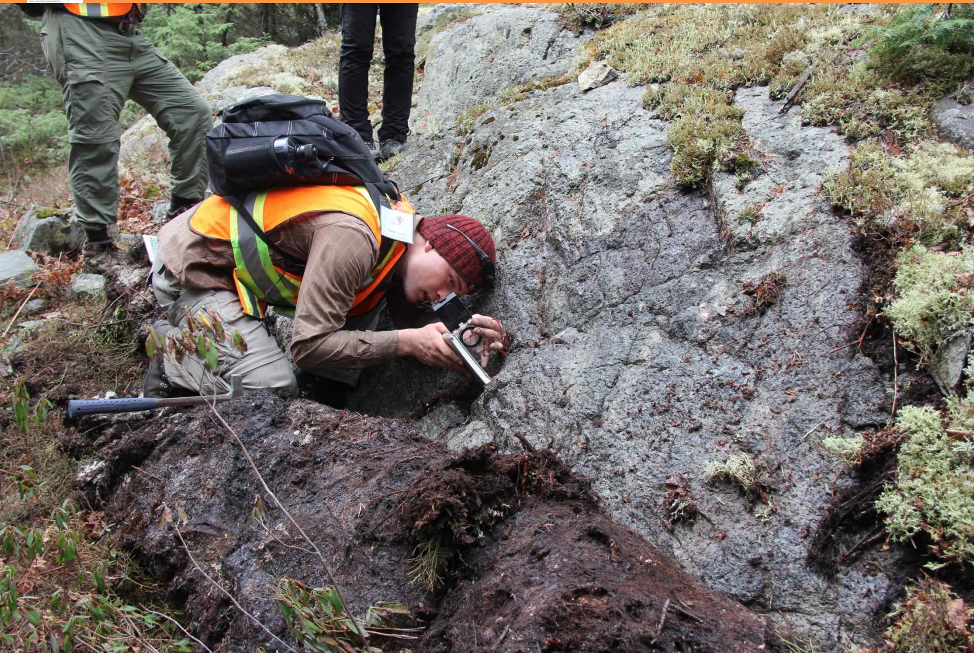
Ryan Bachynski (Regina) measuring the orientation of a vein
