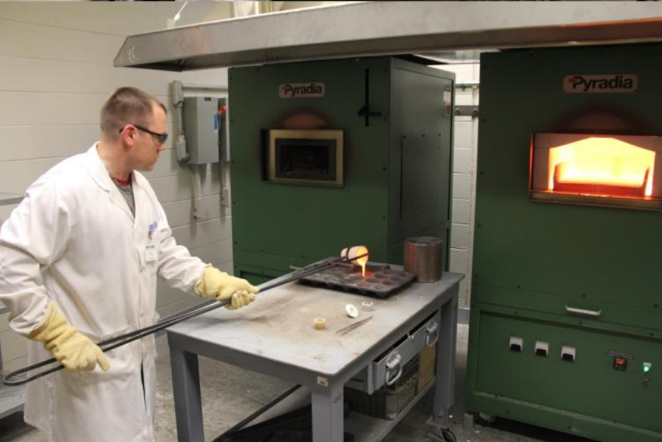
Troy Richardson demonstrates the fire assay technique at the GEOLABS
