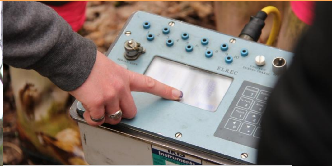
Multi-collector switch box collecting the raw survey data
