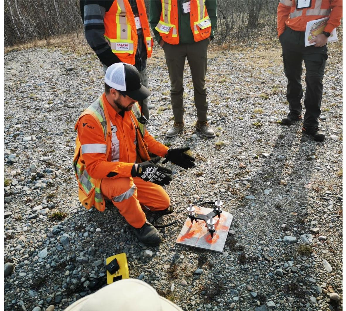
Court Bowers (Vale) shows students the levelling apparatus for the magnetometer.
