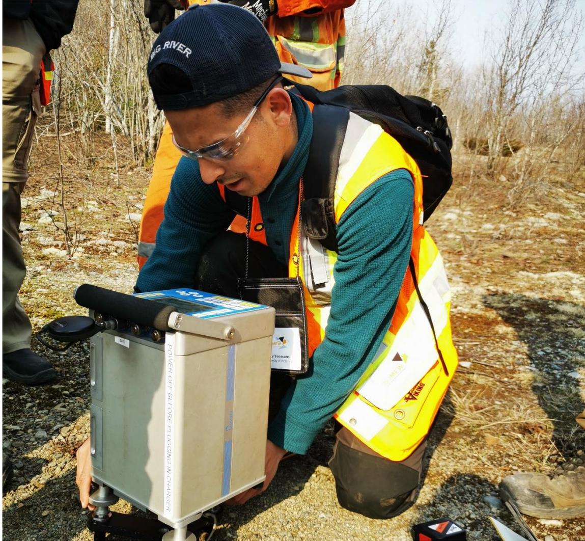
Billy (University of Victoria) levelling the gravimeter for a gravity survey.
