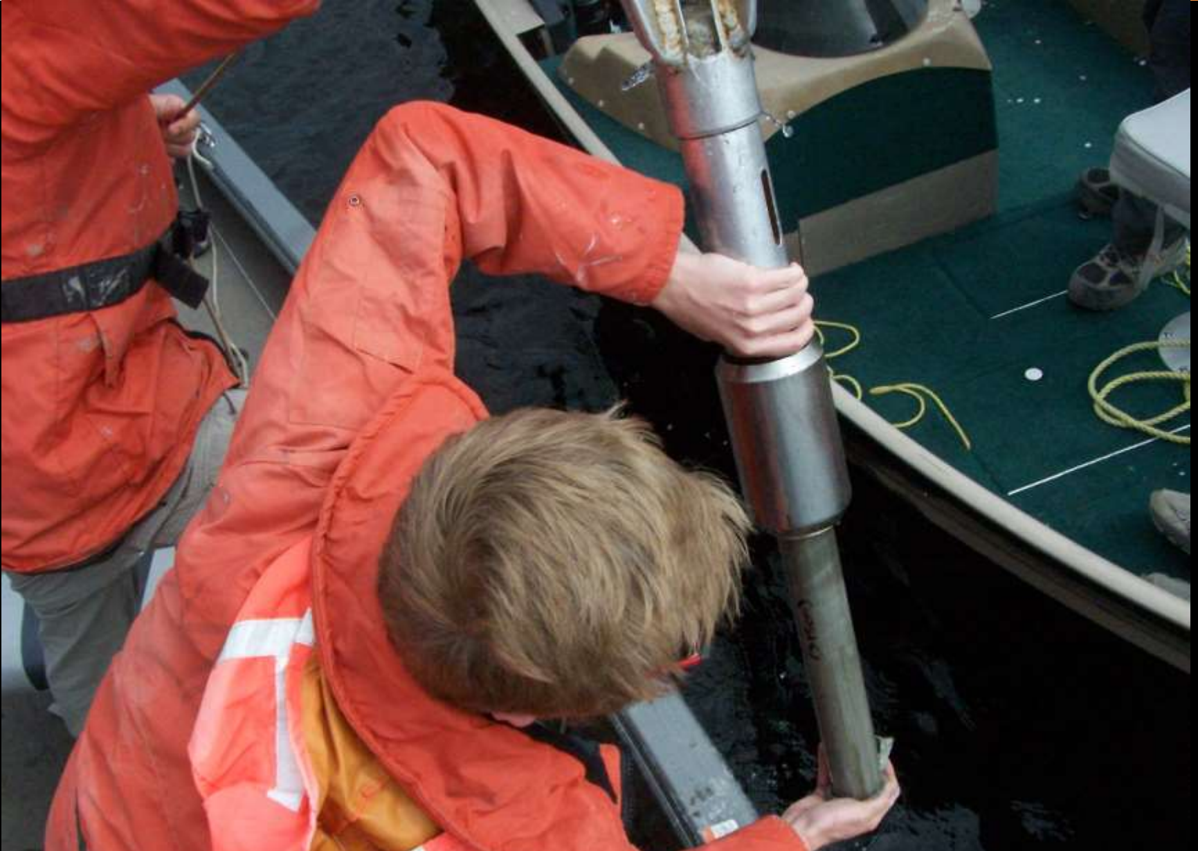
Kurtis Sanderson (University of Victoria) catches a lake sediment sample as it is coming out of the sampling device during Geochemistry Day
