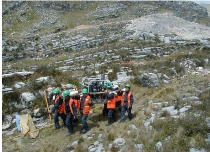
Figure 14: Mobilizing the drill to a high altitude site in Peru. Access roads can be minimized using lightweight, modular drill rigs. © Kluane Drilling
