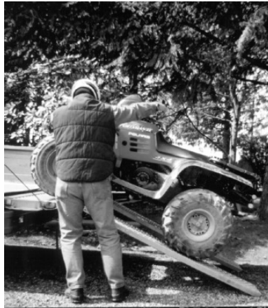
Figure 14.2: The correct way to unload an ATV from the bed of a pickup truck. © Bill Hinde. Used with permission of the Farm and Ranch Safety and Health Association.
