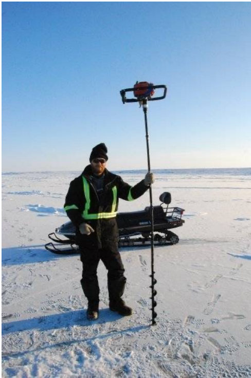
Figure 15.9: Ice auger with extension © Iain Mitchell
