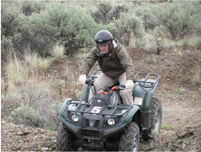
Figure 14.4: Keep weight uphill when descending a slope. © Kim Bilquist
