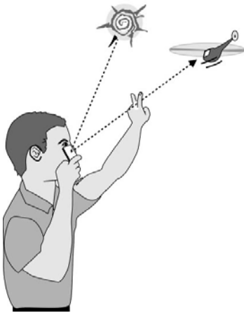
Figure 8.13: Using a signal mirror without a sighting hole
