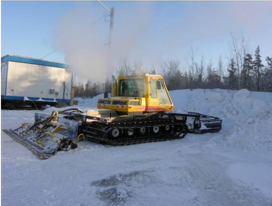
Figure 21.4: Wide tracked Sno-cats are used to clear ice roads and runways on ice. © Iain Mitchell
