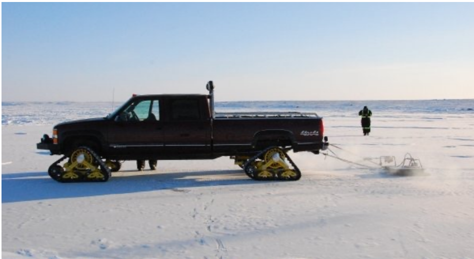
Figure 21.3: Light truck with track conversion towing ground penetrating radar (GPR) ice profiling equipment © Iain Mitchell
