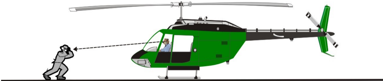
Figure 16.2 Maintaining eye contact with pilot to approach a helicopter.
