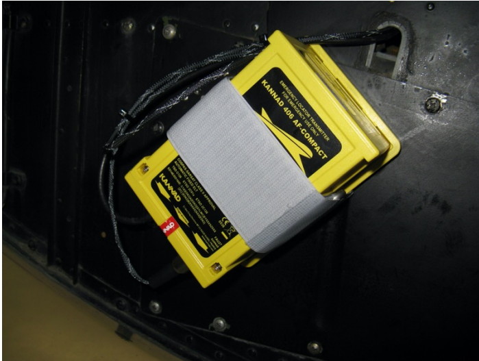
Figure 7.1: 406 MHz Emergency Locator Transmitter (ELT) mounted in a helicopter. © Great Slave Helicopters
