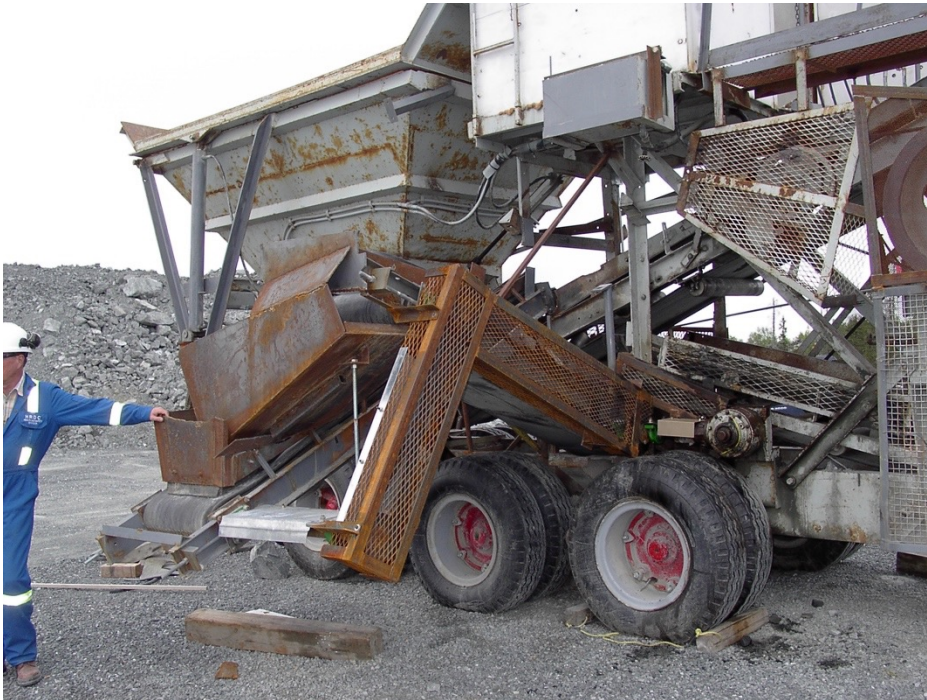
Figure 21.2: Guards and cages protect employees from moving parts of this rock crusher. © Ron Breadmore
