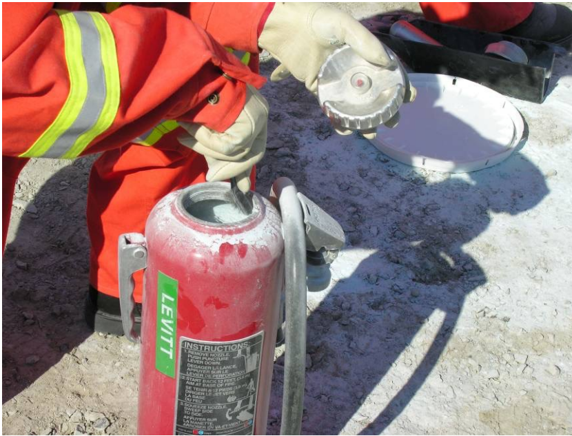
Figure 18.4: Refilling a (BC) fire extinguisher with extinguishing powder (sodium bicarbonate). © Courtney Mitchell
