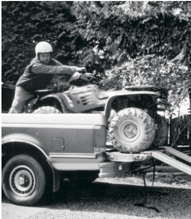
Figure 14.2: The correct way to unload an ATV from the bed of a pickup truck. © Bill Hinde. Used with permission of the Farm and Ranch Safety and Health Association.
