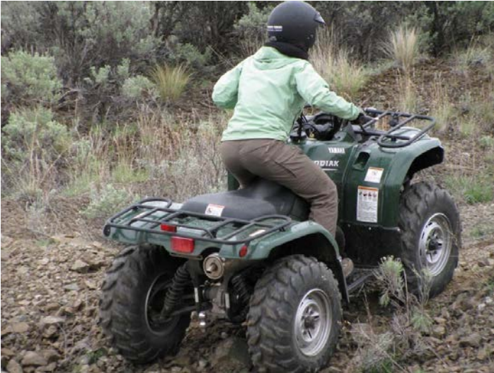
Figure 14.3: Keep weight uphill when ascending a slope. © Kim Bilquist
