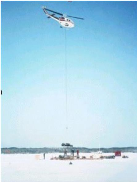
Figure 59: Mobilizing drill rig by helicopter onto Windy Lake. © Wallbridge
