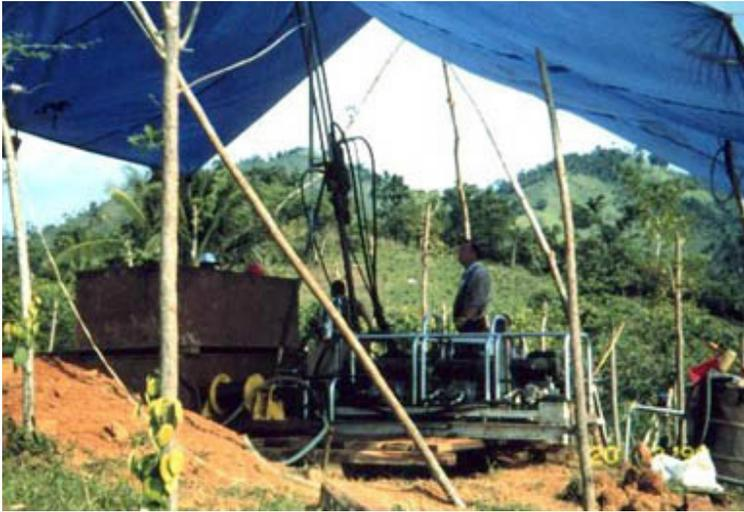
Figure 38: Lightweight, modular drill rigs can mitigate environmental disturbance in tropical terrain. © Kluane Drilling
