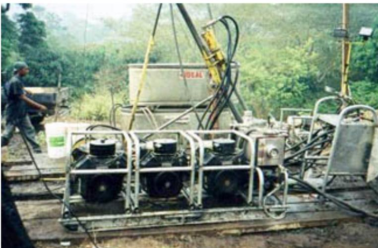
Figure 63: Drill rig showing three tandem engines for increased portability with no loss of power. © Kluane Drilling.
