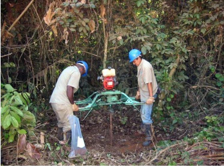
Figure 65: Preliminary exploration (auger drilling) in the rain forests of Carajas, Brazil. © Noranda/Falconbridge.
