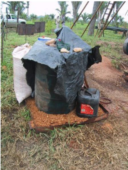
**Figure 42:** Drilling fluids on this project in Brazil are stored on a metal pan filled with wood chips to absorb any drips and spills. The chips can be disposed of safely at the end of the drilling. © Servitec.
