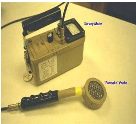
**Figure 47:** Contamination Meter Ludlum Model 12 Pancake G-M Detector\*
