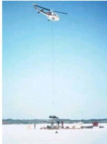
Figure 61: Mobilizing drill rig by helicopter onto Windy Lake. © Wallbridge
