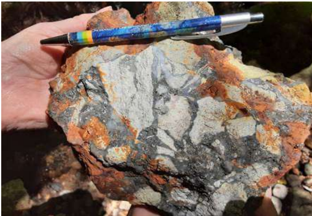
Figure 3: Image of a hydrothermal breccia with silica cement and subangular to angular felsic volcanic clasts with disseminated pyrite.
